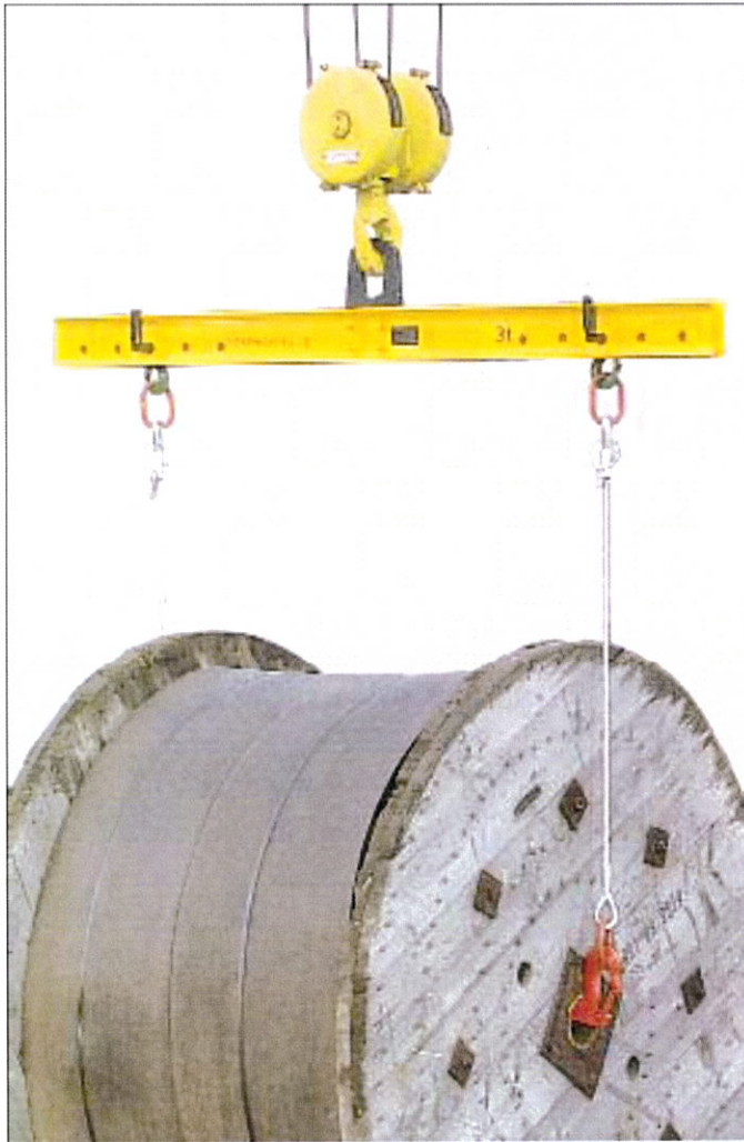
Pic. E3 Loading and unloading of a cable drum by means of a cross arm with straps and cable jaws
