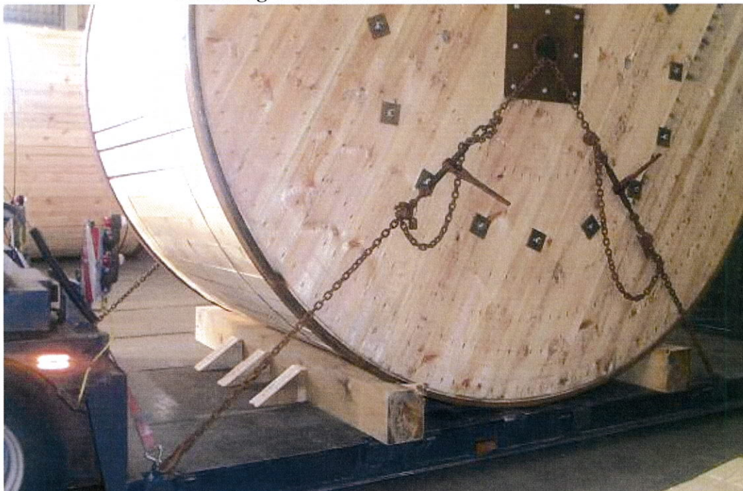
Pic. D1. Fastening of a cable drum to the platform with chains passing through the axis
