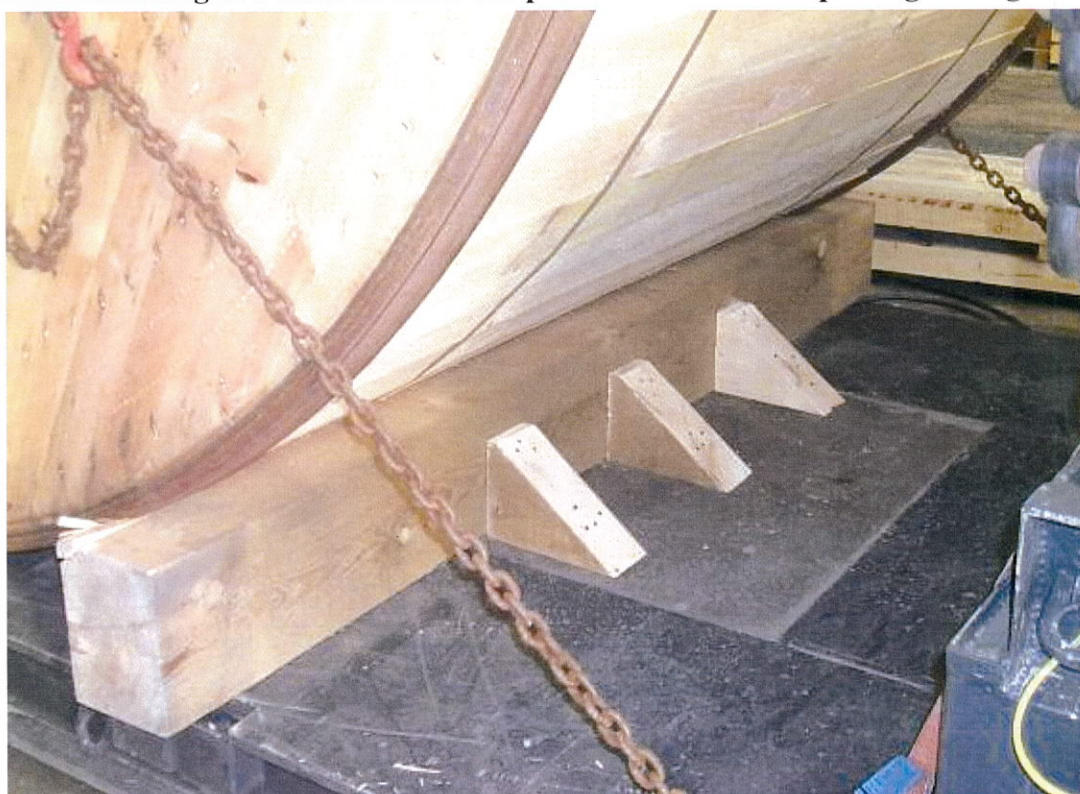
Pic. D2. Fastening of cable on the platform with wooden bars and supports to prevent rolling down
